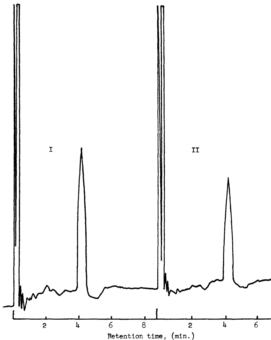
Figure 1. Gas chromatograms of derivatized 4-aminopyridine standard (I) and derivatized purified residue of actual sample-derived 4-aminopyridine (II). (The sample had contained approximately 0.05 ppm of 4-aminopyridine.)
